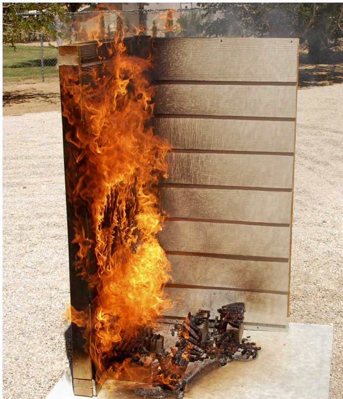
Figure 17. This corner section was constructed with a wood-composite siding material (left side) and a noncombustible fiber cement product (right side). The ignition source for both was a burning brand. The wood-composite siding product was ignited by the ignition source, and the fire then spread up the wall. Flames from the fire would have impinged on windows and eave, if they had been present. The wood brand burned out at the base of the fiber cement siding product without causing significant damage. Photo: Stephen L. Quarles.
