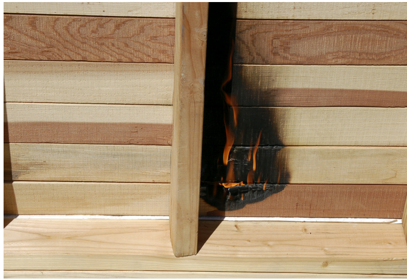
Figure 18. Flame penetration ( burn through ) at the rabbeted bevel lap joint in a solid wood siding product, as viewed from the stud cavity side of the wall. This test was conducted at the UC Fire Research Laboratory. Although a panelized sheathing product is commonly used in construction, it was not used in this test in order to allow viewing of the siding performance. Use of sheathing has been shown to increase the time needed for fire to penetrate into the stud cavity, sometimes to the point of excluding entry altogether. Photo: Stephen L. Quarles.
